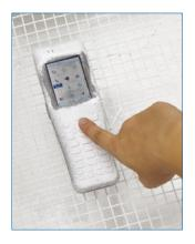
The DT-X8 is shock protected against drops from a height of up to 3 metres onto concrete. This completely covers allimpacts and fall heights that typically occur in a warehouse. The terminal withstands dust and temporary immersion in water in accordance with protection class IP67 and it works at temperatures down to -20°C. This guarantees that the device can be used outdoors the whole year, as well as in cold stores, wet areas and in particularly dusty or dirty environments.
