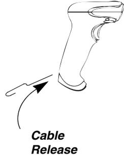
6. Replace with the new cable. Insert the connector into the opening and press firmly. The connector is keyed to go in only one way, and will click into place.
